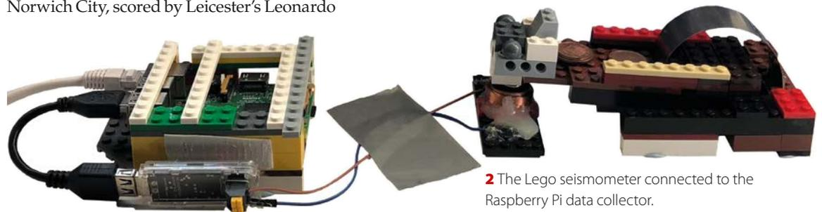
**2** The Lego seismometer connected to the Raspberry Pi data collector.
